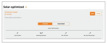
If the consumption strategy for devices is to be a combination of solar optimization and time control, the EnergyManager Portal also offers the option of defining time periods in which solar optimization is compulsively deactivated.
